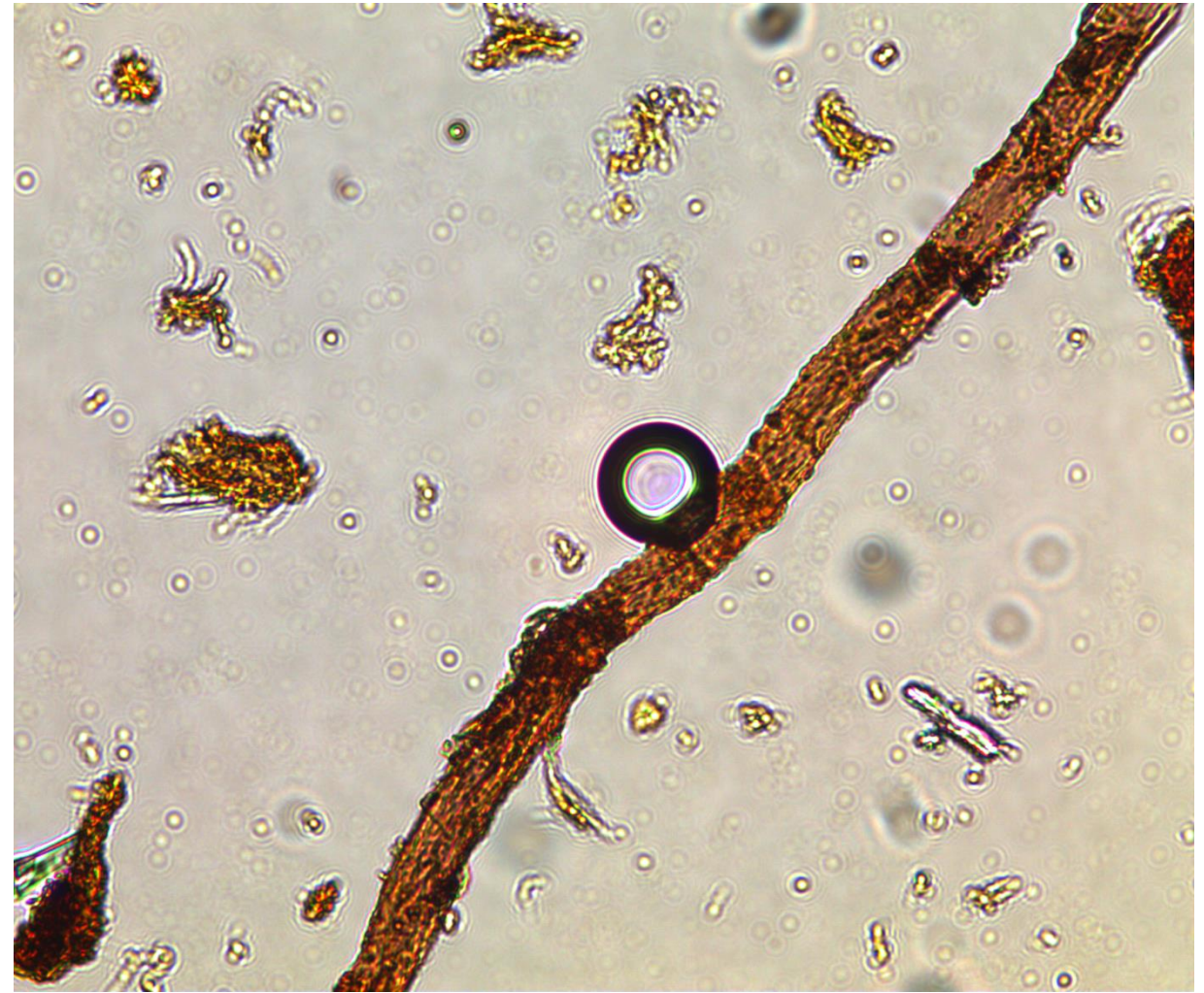
Photomicrograph of colonial currency from 1759 of flax at 400X, stained with Graff "C" stain.
