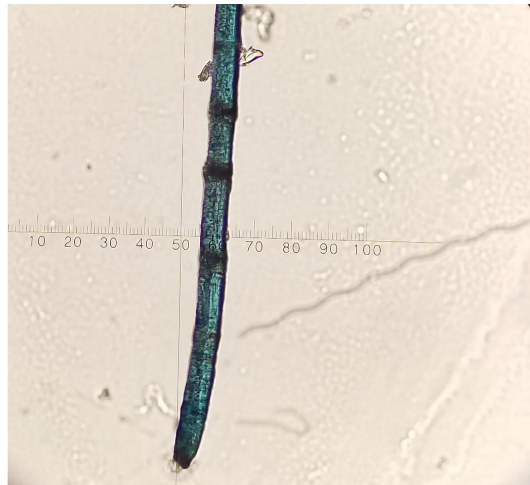
Photomicrograph of dyed blue fiber of colonial currency from 1775 of flax at 200X.
